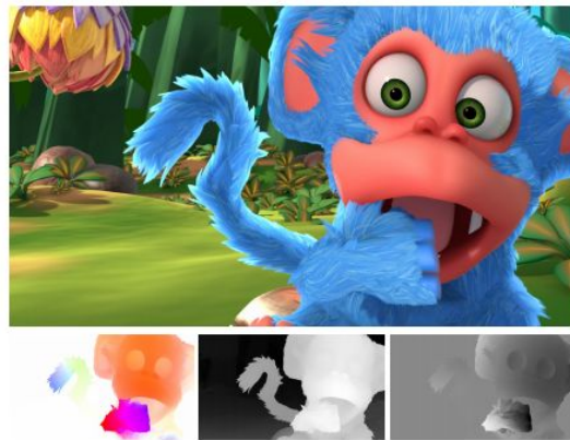
Figure 1. Our datasets provide over 35 000 stereo frames with dense ground truth for optical flow, disparity and disparity change, as well as other data such as object segmentation.
